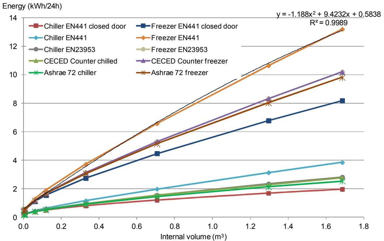
**Figure 7. Graph of energy consumption per 24 hours against cabinet volume for upright cabinets according to different test methodologies, showing results from the mathematical model.**
