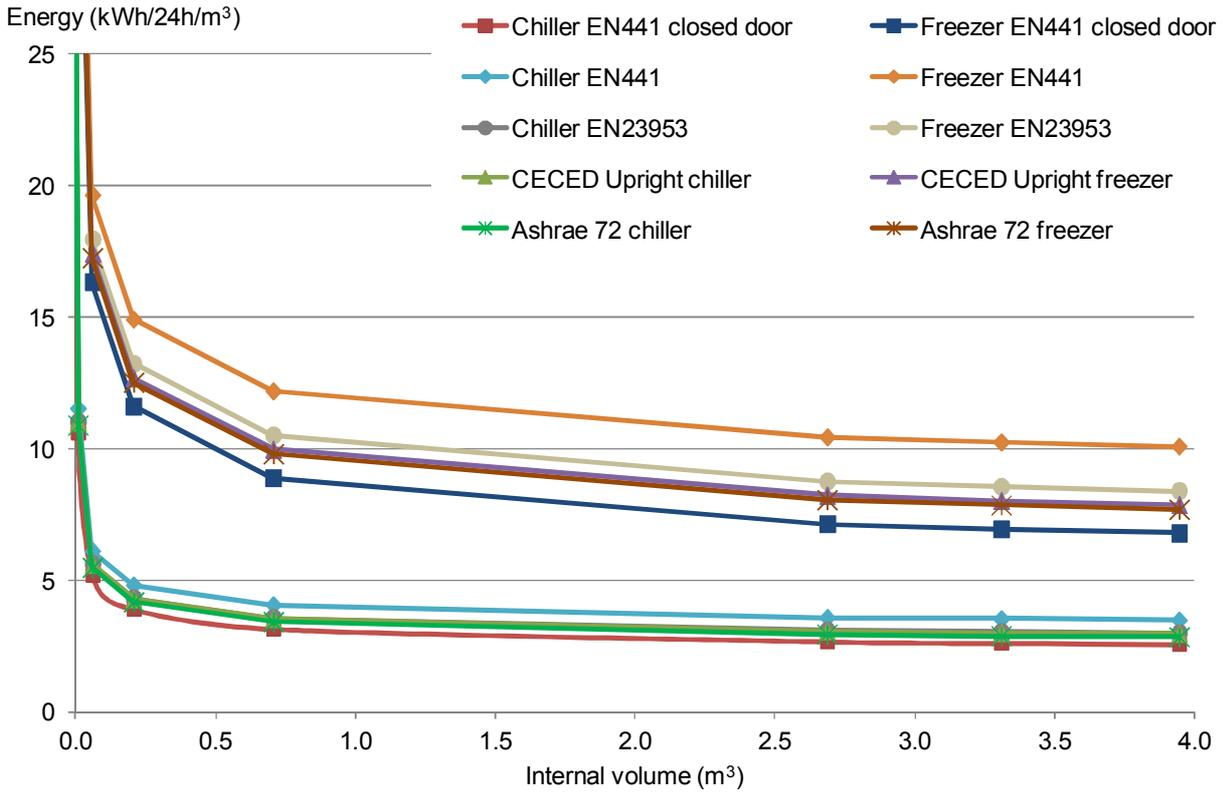
**Figure 4. Predicted energy consumption per cubic metre of net volume for a horizontal cabinet according to the different test regimes.**
