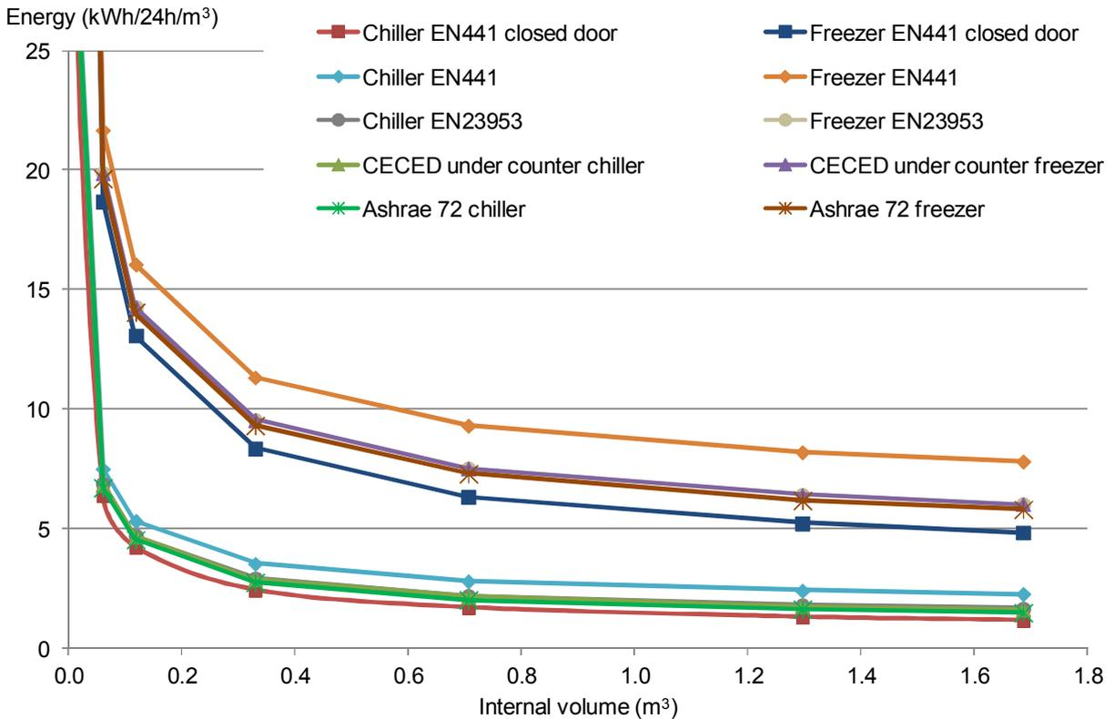
Figure 5. Graph showing how the spread of ASHRAE 72 test data compares to the predicted consumption from the model
