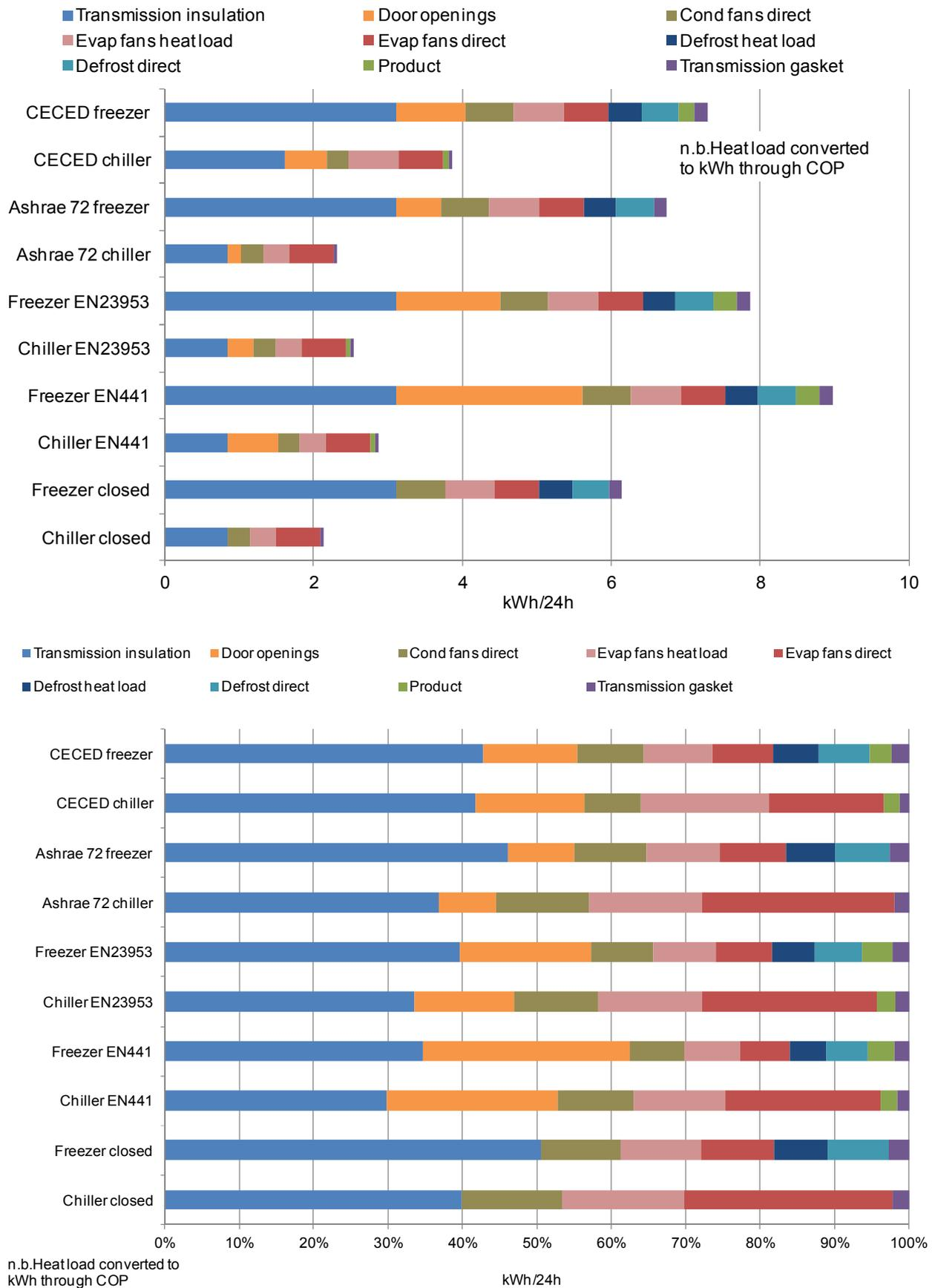
**Figure 2. Model outputs, showing two views of the same data of proportion of total energy consumption for a counter cabinet attributable to certain sources, for freezer and chilled cabinets tested according to various test methodologies. First view in kWh/24hrs, second as a percentage.**
