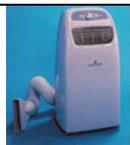
**Single ducts** consist of one single unit placed freely in the room. The air is expelled through a duct, which requires a window to be open. Warm air is drawn into the room, as the condenser is cooled with air taken from the room – the cooling effect is small and only local.
