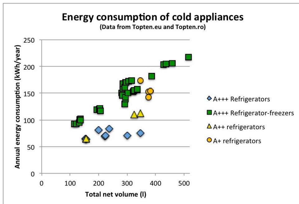
Fig. 4: Declared Energy Consumption of A+++ refrigerator-freezers and refrigerators (A+ and A++ refrigerators for comparison)
