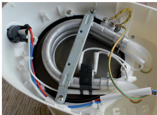
Figure 2. Heating unit of drip filter machine.
